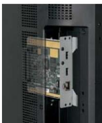
An optional board can slide into the slot on the back of the monitor.
